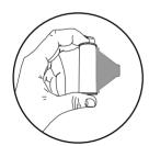
Take your 120 exposed film, open the lid and open the module grey lock. Be sure the 120 knob is in open position (triangle symbol).
