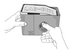
Push the grey lever upwards on the back to release the film from the cartridge.
