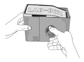
Close the lid and turn the outer knob in order to wind the film onto the reel.
