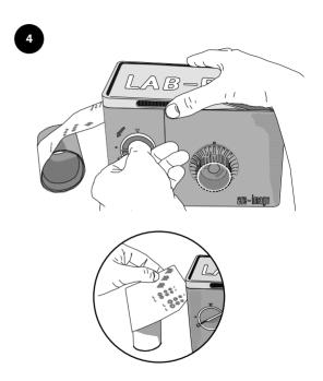
Turn the 120 knob counter-clockwise into closed position (square symbol). Now you can tear away the paper.
