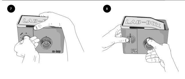
Close the lid and turn the 120 knob (triangle position) to open the lightproof chamber and release the film.
