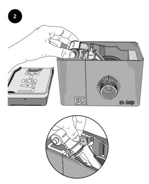
Open the lid and place the roll in the film slot. Then slide the film under the two metal pins.
