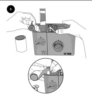
Open the lid and carefully remove the spool. Pay attention to not pull out the film. Remove the excess backing paper and the adhesive from the film.
