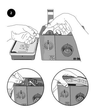
Feed the black backing paper through the rear slit and place the roll in the film slot. Close the grey lock as well as the lid.
