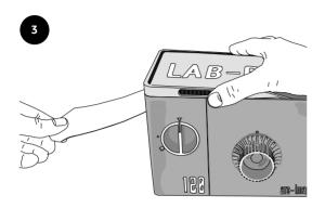
The film will be automatically wound into the lower lightproof chamber behind the 120 knob.
