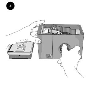
Turn the outer knob until the hooked film starts to slide correctly though the film guide.
