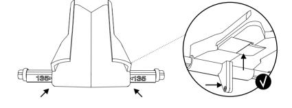
Check that the 135 reels are in the correct position and properly aligned. Follow L, R and the arrow indicators on the reels and the hub as a reference.
