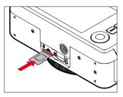
Push the memory card into the slot with the contacts pointing towards the lens until you hear and feel it clicking into place
