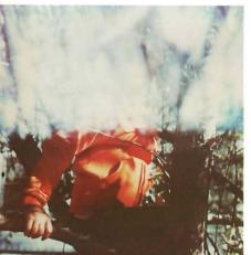
Part of the picture is fogged: If you press against the bellows while taking a picture, you may block the movement of parts inside the camera. The next picture you take could be partially or totally white or could have streaky light patterns.
