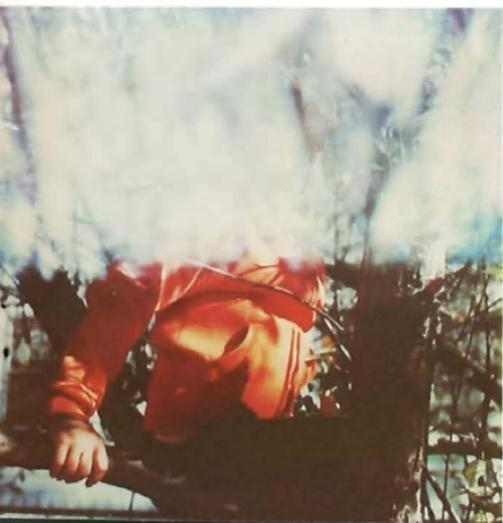
**Part of the picture is fogged:** If you press against the bellows while taking a picture, you may block the movement of parts inside the camera. The next picture you take could be partially or totally white or could have streaky light patterns.
