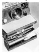
The rollers inside the film compartment should be kept clean. Before loading each new pack of film, examine the rollers by rotating each one separately.
