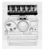
Insert a FlashBar into the socket on the top front of the camera body above the lens or sonar and push in firmly.
