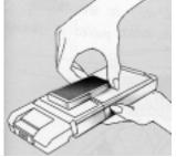
Hold the camera in the palm of your left hand. Grasp the sides of the viewfinder cap at the rear (ribbed surfaces).
