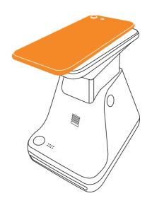
04 **Close the film door.** The darkslide will eject automatically beneath the film shield. Lift the film shield and allow it to roll back up, then remove the darkslide.
