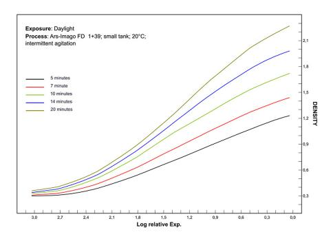
Sinuous-looking curve, with an extended toe that lessens the effects of underexposure yet generally giving back deep shadows and good details, especially when working with a slight overexposure. The image's overall tone is balanced with particular emphasis on darker tones.
