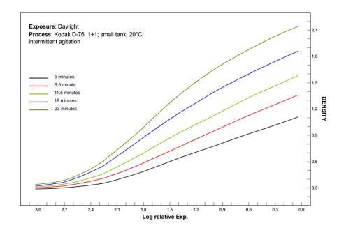
This curve is characterised by a short toe and a good contrast if exposed correctly. The portion tends to raise, emphasizing the midtones and the mid-high tones that are through slightly lighter tones than normal and returning images that tend to be more open and airy.
