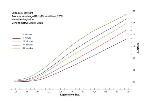
Rectilinear curve with a short toe and without a hint of a shoulder on the lights; excellent tone separation both on the tone scale extremes and on the midtones, with a highly linear contrast reproduction.
