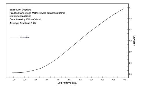
The curve trend is regular and rectilinear, indicating a good and firm tone separation. Contrast on the negative is generally high; a good print can be obtained by using a multigrade contrast filter n. 1.
